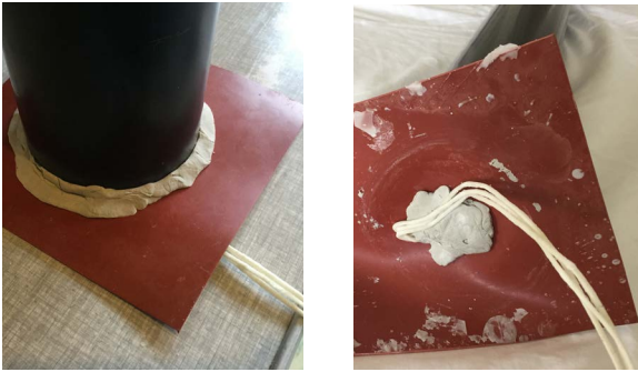
Creating the bottom seal with a rubber gasket and putty.
