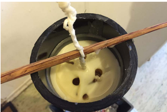
Holes created with a dowel to pour more wax into the inside.
