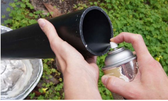
Spraying candle release spray into the mold tube.
