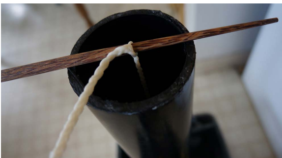
Holding the wick with a chopstick at the top of the mold.
