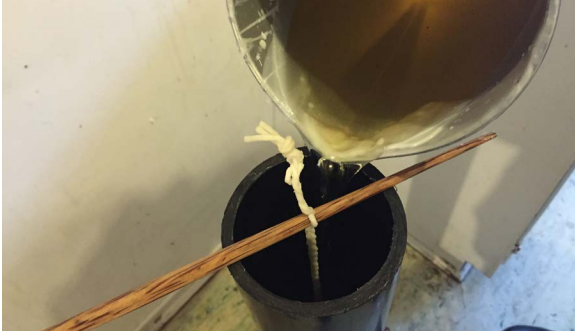
Pouring almost all the wax in the first pour.
